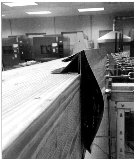
RE-2 testing being conducted on fascia.
